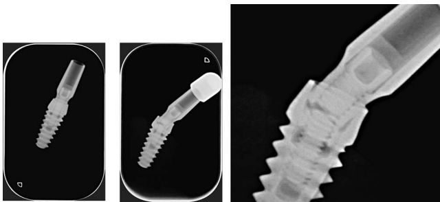
FIGURE 6. Group I: radiograph evaluation of the conometric joint implant tested. Left: Prior fracture strength test. Middle: after the loading. Right: detail of the implant-joint connection after the test.
