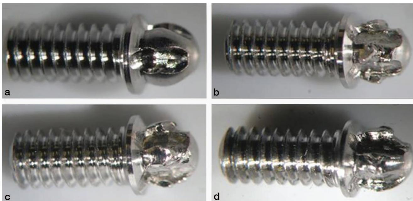
**FIGURE 2.** Deformed Ball Head System screw grooves. (a) Nontested screw. (b) Screw tested at 0°. (c) Screw tested at 20°. (d) Screw tested at 30°.
