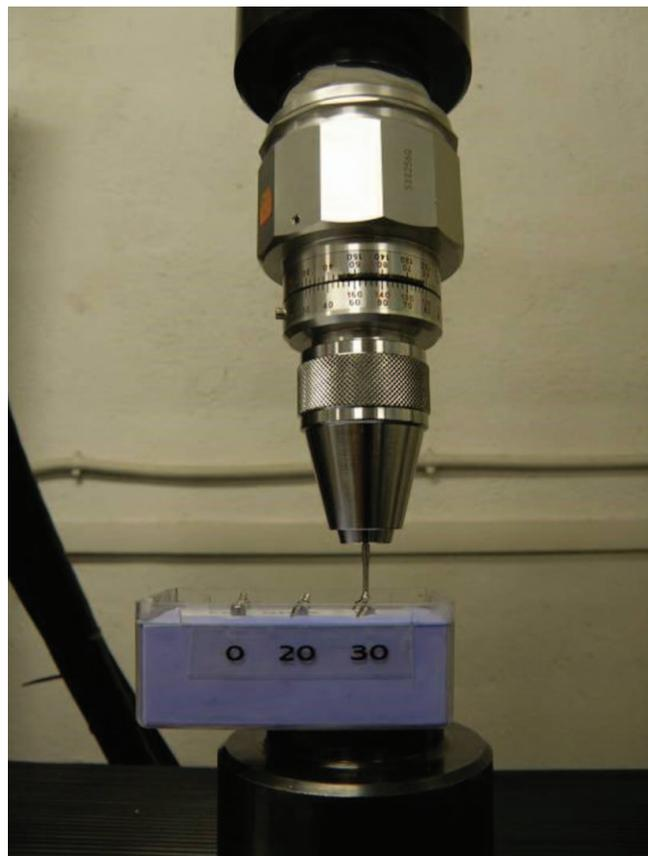
**FIGURE 1.** Analogue torque meter. Assembly of the analogue torque meter for the test set.
