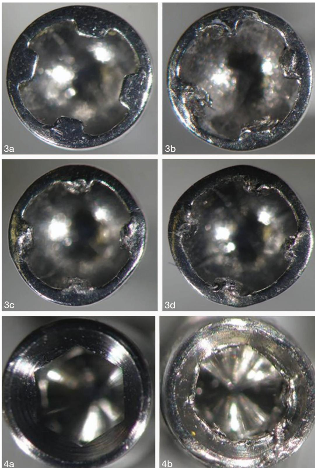
**FIGURES 3 AND 4. FIGURE 3.** Inner aspect of the Ball Head System (BHS) screwdrivers. (a) Nontested screwdriver. (b) Screwdriver tested at 0°. (c) Screwdriver tested at 20°. (d) Screwdriver tested at 30°. **FIGURE 4.** 1.3-mm hexagonal screwdriver system. (a) Nontested screw. (b) Tested screw.
