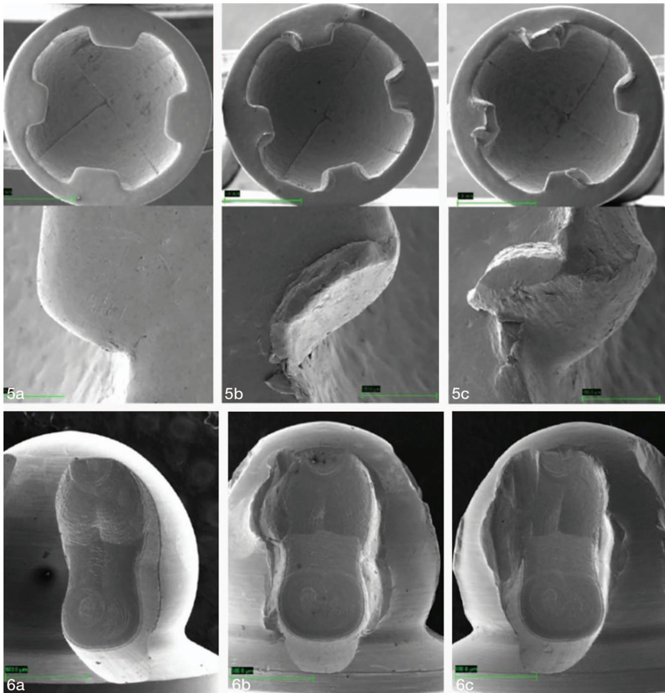
**FIGURES 5 AND 6.** **FIGURE 5.** Ball Head System (BHS) screwdrivers visualized by field emission scanning electron microscopy (FESEM). Upper bars show 1.0 mm and lower show 150  $\mu\text{m}$ . (a) Nontested screwdriver. (b) Screwdriver condition after 10 iterations. (c) Screwdriver condition after 30 iterations. **FIGURE 6.** BHS screws visualized by FESEM. Bars show 500  $\mu\text{m}$ . (a) Nontested screw. (b) Screw condition after 10 iterations. (c) Screw condition after 30 iterations.
